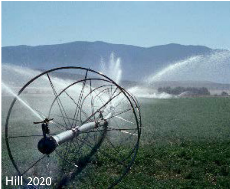
High-pressure impact sprinkler
